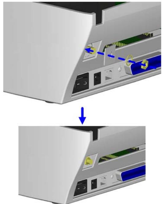
12. Screw the antenna onto the antenna connector. You can now adjust the angle of the antenna as required.
