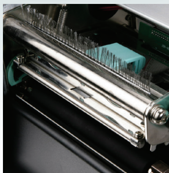
Easy to change, low-cost printhead assembly
